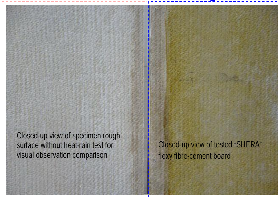
Fig 7: Visual observation of specimen rough surface installed facing outside test chamber after after heat-rain test.
