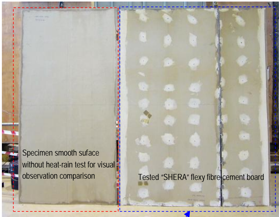
Fig 7: Visual observation of specimen smooth surface installed facing inside test chamber after exposed to 50 cycles of simulated heat-rain.
